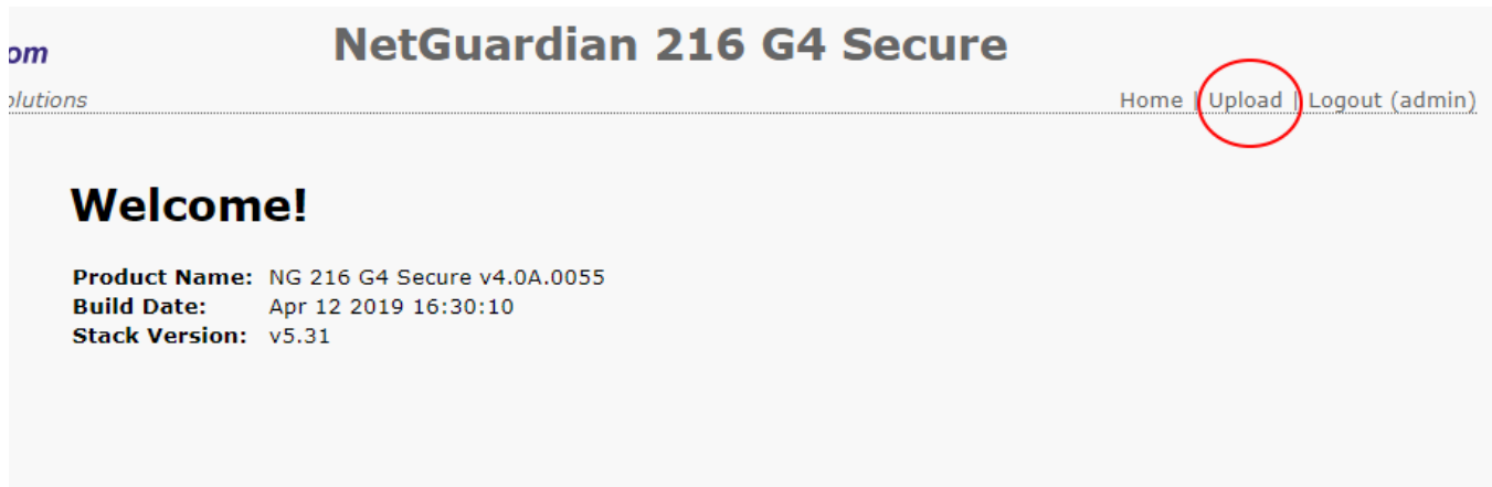
Fig. 14.1 To upload firmware, click on Upload on the top right corner of the web interface
