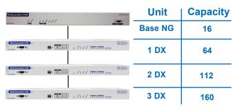
The NetGuardian 864DX G5 is another option to achieve discrete and analog expansion. Each chassis adds 64 discrete alarm points, providing a total of **208** when 3 NetGuardian 864DX G5 units are daisy-chained.
