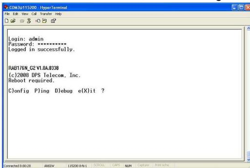
16. When prompted, enter the default user name **admin** and password **dpstelecom**. **NOTE:** If you don't receive a prompt for your user name and password, check the Com port you are using on your PC and make sure you are using the cable provided. Additional cables can be ordered from DPS Telecom.
