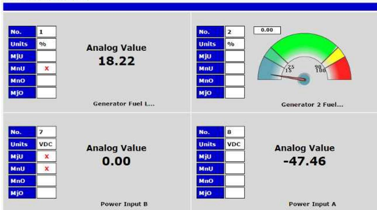
*Fig. 12.6* Current status of all analog inputs in the Monitor > User Analogs in Gauge View.
