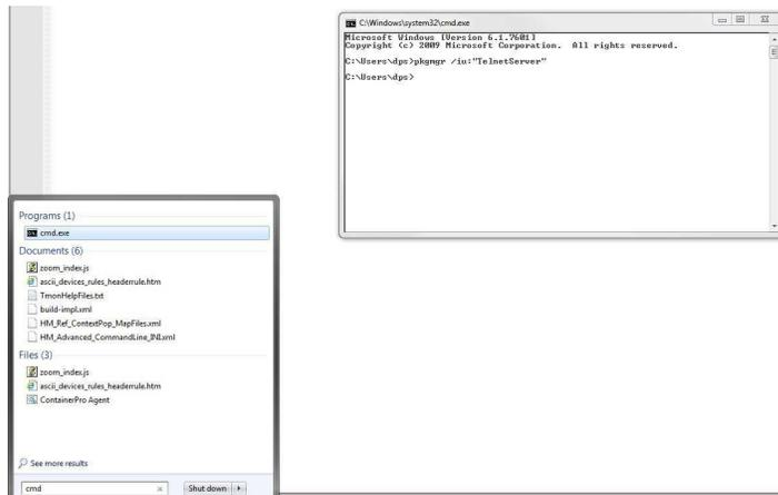
From the command line, type in **pkgmgr /iu:"TelnetClient"** then press **enter**. When the command prompt appears again, the installation is complete.
