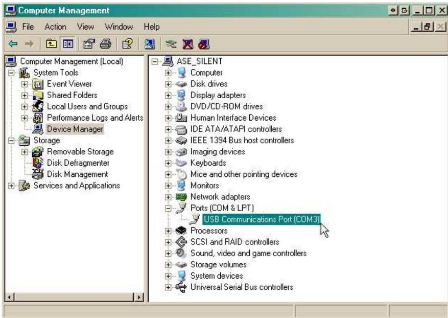
11. Expand the "Ports (COM & LPT)" section in the right pane. Look for "USB Communications Port (COMx)". Note the number of the COM port ("COM3" in the example above).
