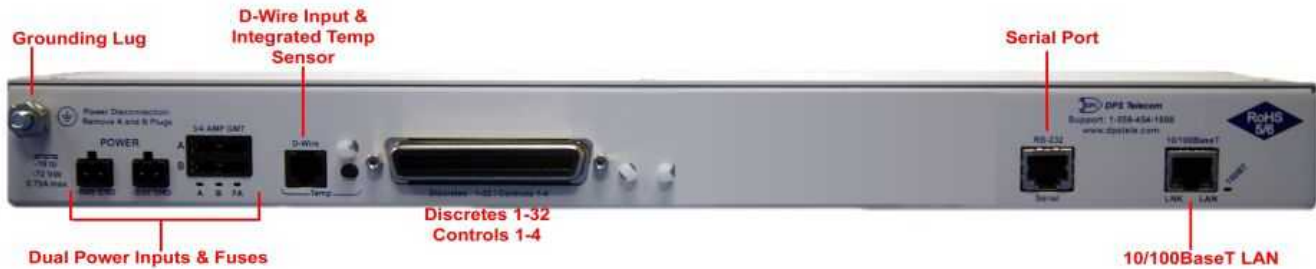
NetGuardian 432 G3 back panel connections
