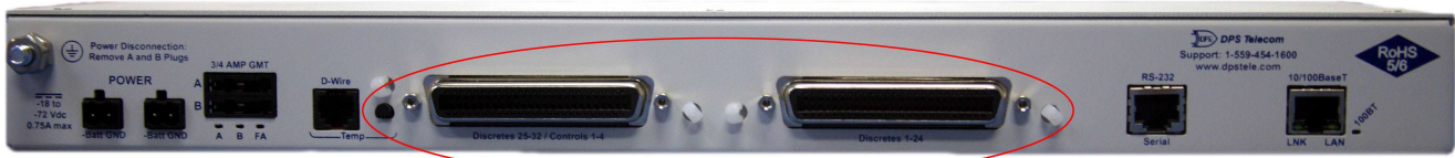
NetGuardian 432 G4 Alarm and Relay Connectors
