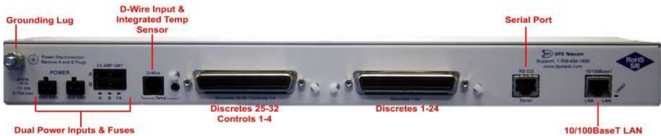
NetGuardian 432 G4 back panel connections
