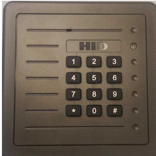
5. Loosen the four screws to open the enclosure (the enclosure screws are captive in the cover).
