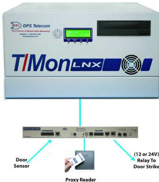
*In the Building Access System, the NetGuardian ENV operates independently of an RTU*
