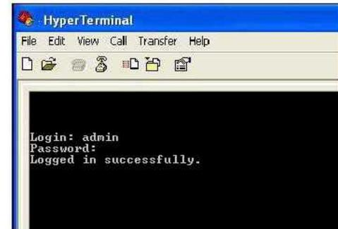
6. The NetGuardian ENV's main menu will appear. Type C for C)onfig, then E for E)thernet. Configure the unit's IP address, subnet mask, and default gateway.
