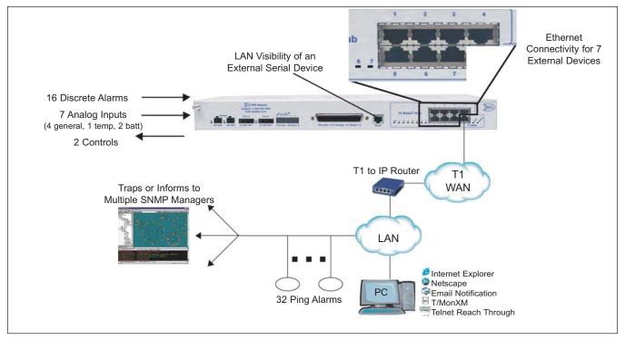
In addition to LAN, the NetGuardian 216T supports FrameRelay/T1, providing detailed monitoring and Ethernet connectivity at remote sites. It also supports remote Telnet connections to an external serial device.
