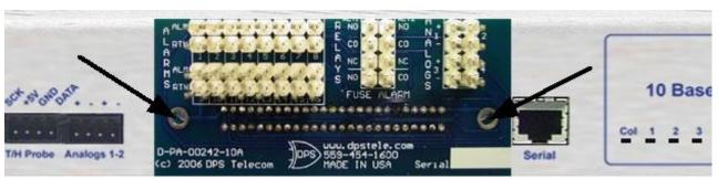
Fig. 6.7.1. The wire-wrap back panel (arrows indicate screw locations for mounting)
