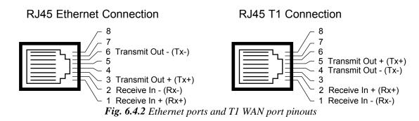
The pinouts for the Ethernet hub ports and the T1 WAN port are shown in Figure 6.4.2, above.
