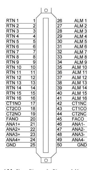
Fig. 6.5.2.. Pinout Diagram for Discretes 1-16 connector
